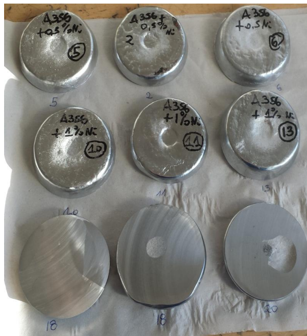
Figure 2 - Specimens for GD-OES analysis.
