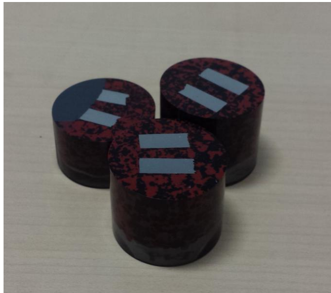
Figure 10 – Samples for microstructural analysis showing the fracture profiles of the tensile specimens.
