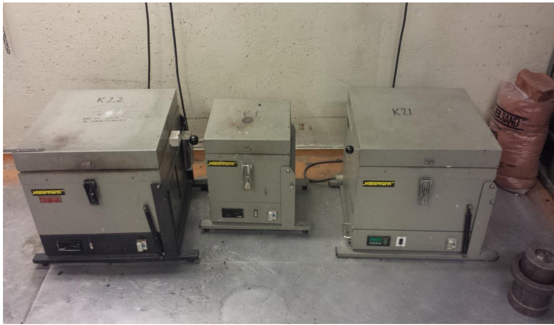
Figure 1- The melting furnaces used for the experimental work
