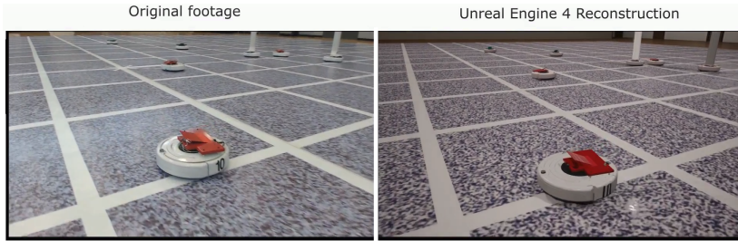
Figure 3.4: A dataset containing 1089 images was made in Unreal Engine 4 to perfectly mirror a real-world dataset containing Roomba vacuum cleaning robots inside a gym arena. Even though the two datasets were completely similar, a CNN (YOLO [23]) trained on the synthetic domain to detect Roombas, did not perform well in the real-world domain, showing computer graphics contain features building up to a dataset bias. However, some overfitting were present in the experiment.
