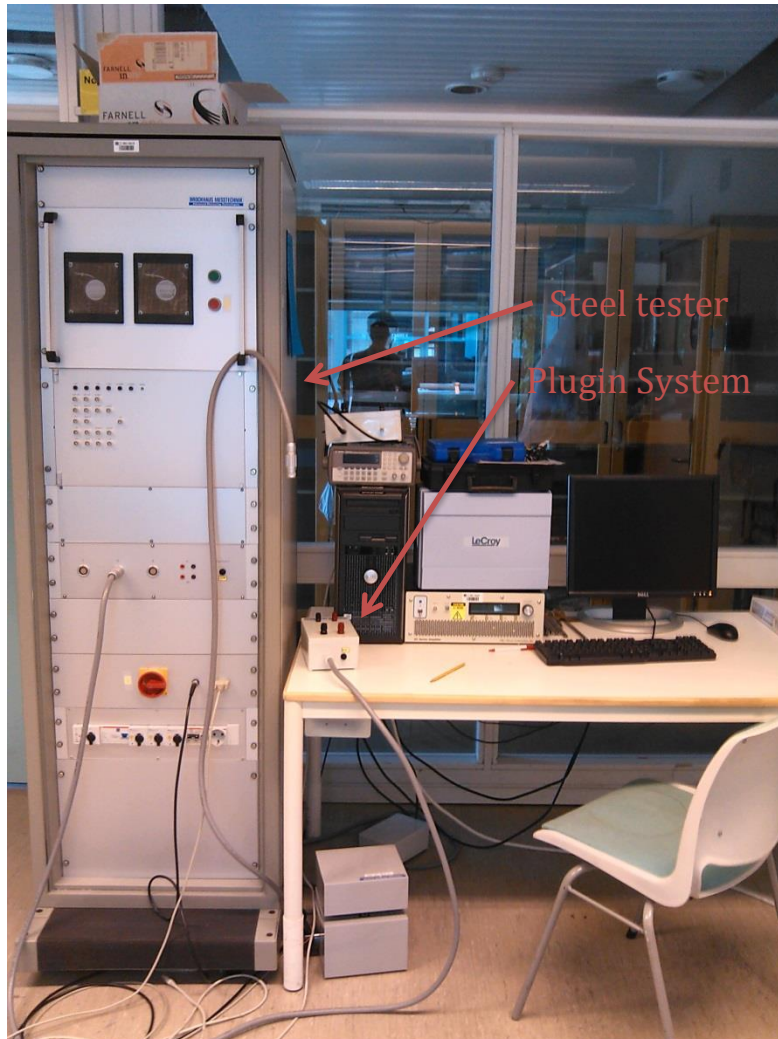
Figure 13-4 The loss measurement setup with a Brochause steel tester
