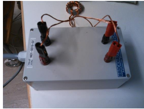
Figure 10-3 The plugin system for ring cores in BROCHAUS MPG 100D
