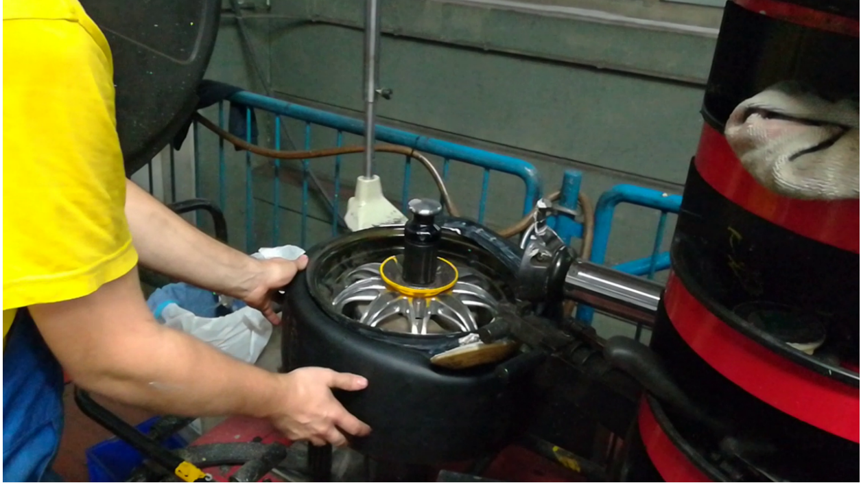
Figure 3.5.9: Tire changing performed with a tire changing machine
