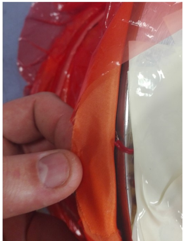
Figure A.8.8: Left: Bagtape rolled in release film, used to reduce bridging around bead. Right: Temperature sensor, mounted between mold and laminate
