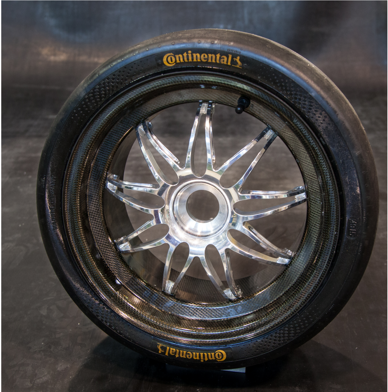
Figure 3.4.2: Final assembled wheel
