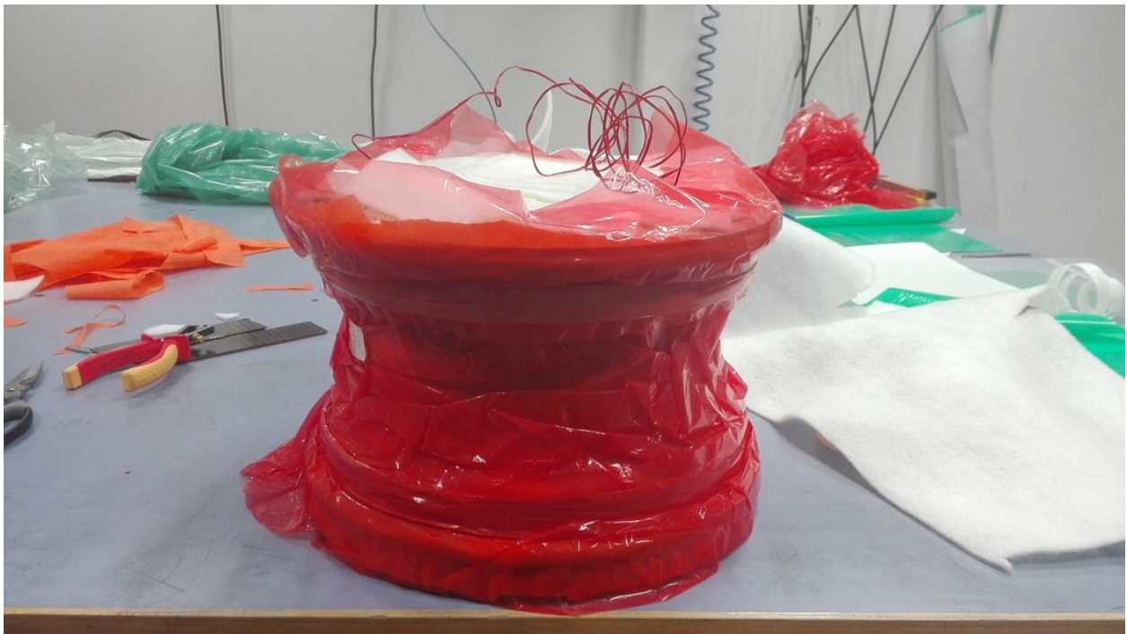
Figure A.8.9: Finished application of release film
