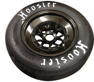
Figure 1.3.1: 2-piece concept, Revolve NTNU 2014 [4]
