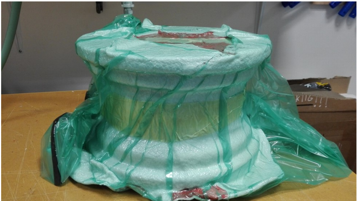
Figure A.8.5: Rim shell under debulking
