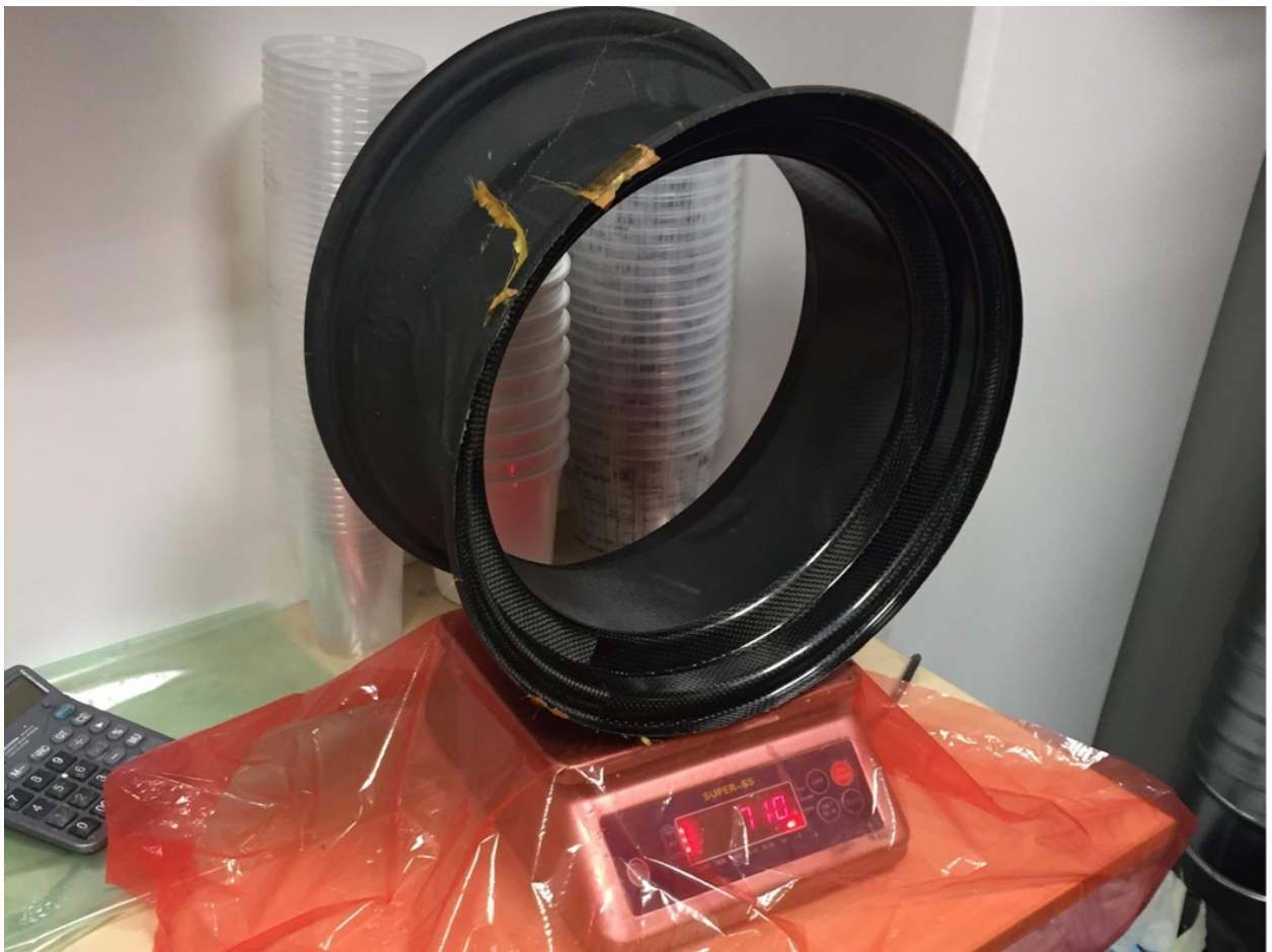
Figure A.8.20: Finished cured and demolded rim shell, here on a scale for controlling the weight
