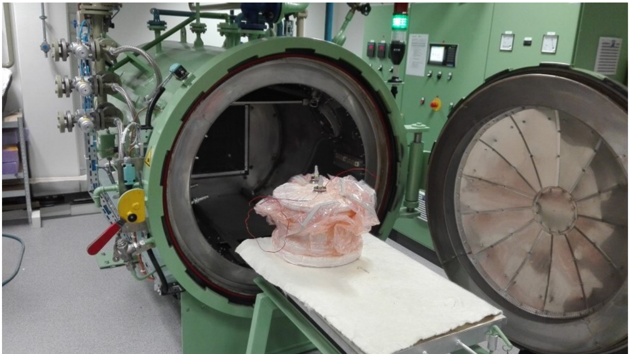
Figure A.8.13: Rim shell ready for autoclave curing
