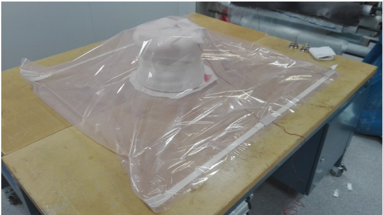
Figure A.8.11: Vacuum bag ready for sealing
