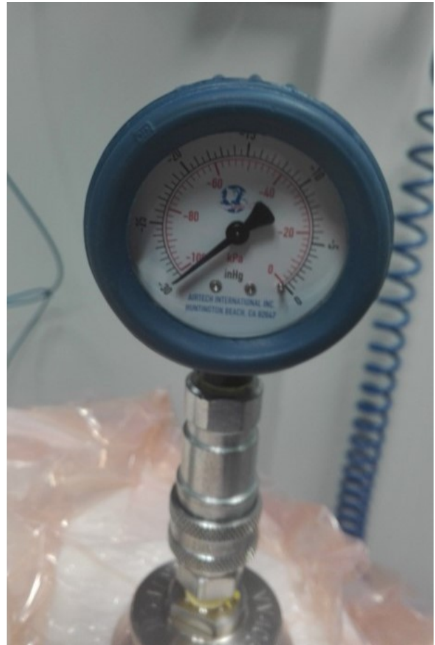
Figure A.8.12: Vacuum leak test
