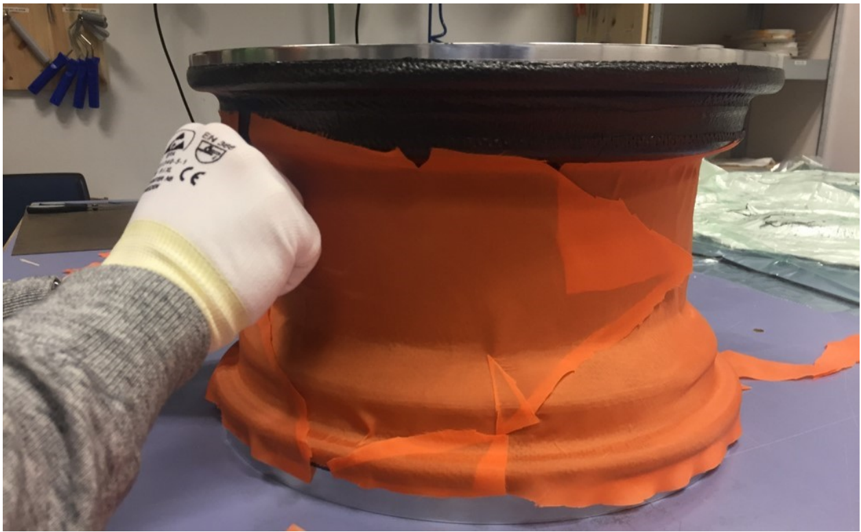
Figure A.8.7: Application of peel ply
