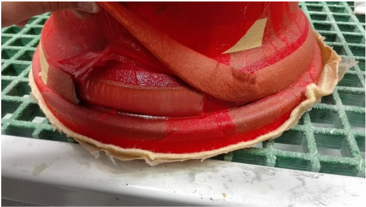
Figure A.8.17: Removal of release film
