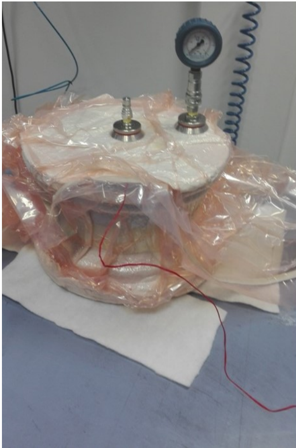
Figure A.8.12: Vacuum leak test
