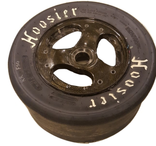
Figure 1.3.4: 2-piece full CFRP concept, Revolve NTNU 2016
