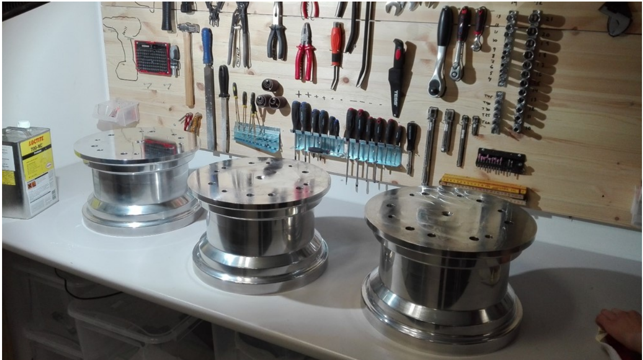
Figure A.8.1: Molds after polishing, application of sealer and release agent.
