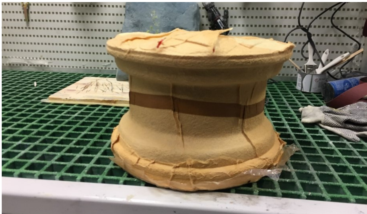
Figure A.8.16: Rim shell under demoulding
