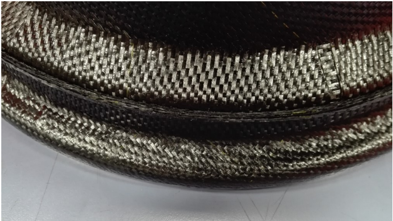
Figure A.8.6: The hump was created by stacking small stripes of CFRP
