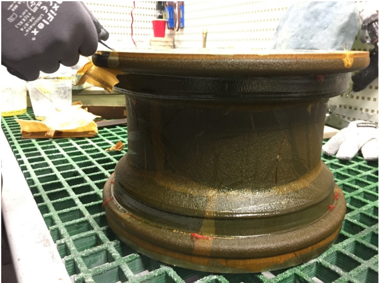
Figure A.8.18: Removal of peel ply before demoulding
