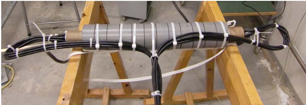
Figure 4-6: Picture of small transformer with a long no-loop secondary winding
