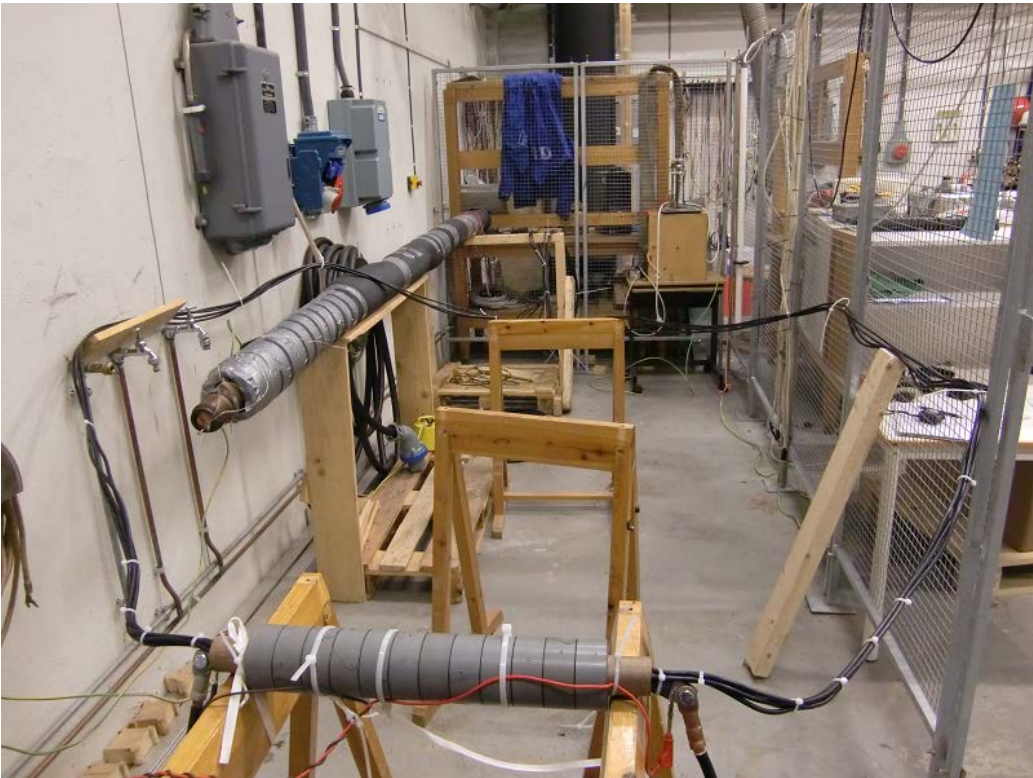
Figure 13-4: Picture of small transformer with a long half-loop secondary winding
