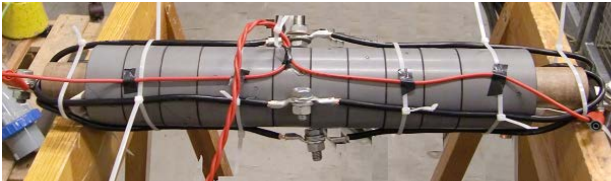
Figure 4-3: Illustration of twisted voltage measurement conductors, small transformer
