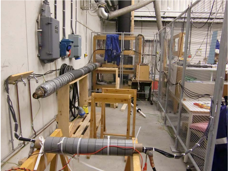
Figure 13-5: Picture of small transformer with a long full-loop secondary winding
