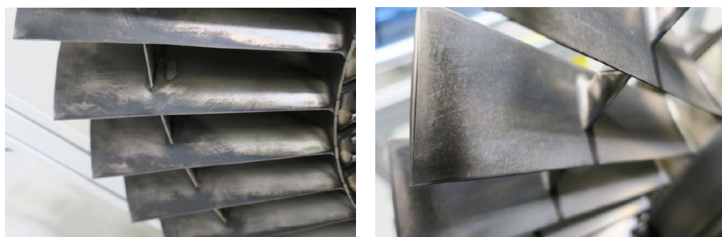
Figure 36. HPC stage 1 rotor blade SS (left), stage 1 rotor blade PS (right) [9]
