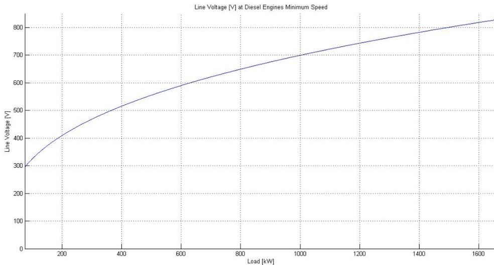
**Figure 40** Line voltage at diesel engines minimum speed
