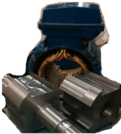
Fig. 21: Photograph of the stator and rotors before magnets were attached.
