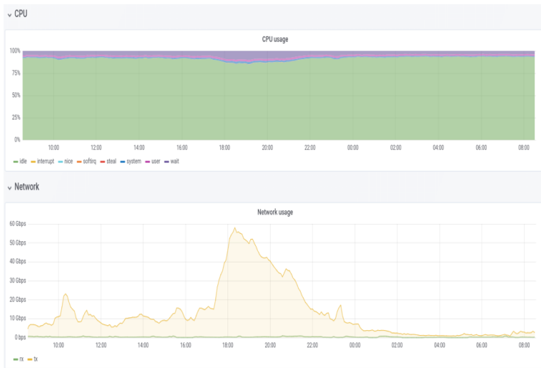
Figure 2.1: Average CPU and Network utilization on the ALICE EOS cluster. Idle CPU shown in green.
