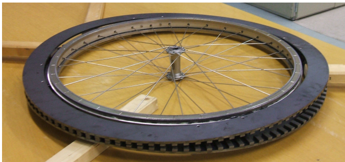
Fig. 8. Collapsed rotor. The magnets touch each other at the left front and right back of the picture, and are pushed 5 cm away from each other at the right front and left back.
