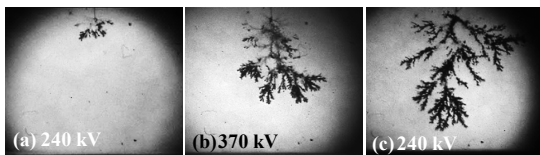
Figure 23. Typical shapes of the negative 1 st mode streamers; (a)-Neat white oil; (b)-Neat white oil; (c)-Neat white oil at reduced pressure.
