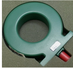
Figure 7.4 Pearson current Probe
