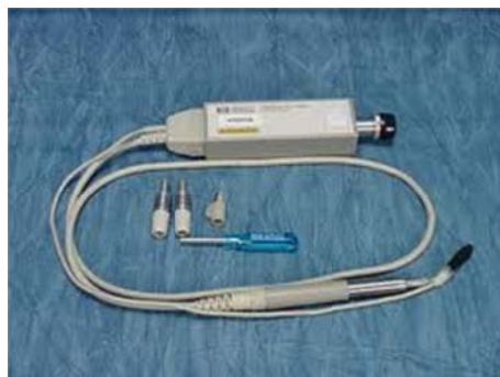
Figure 7.3 Agilent 41800A series active Probe
