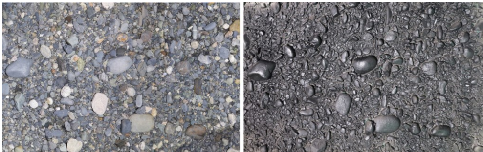
Fig. 2. Left: Water-worked gravel surface, Right: Non-porous counterpart of gravel (cast)
