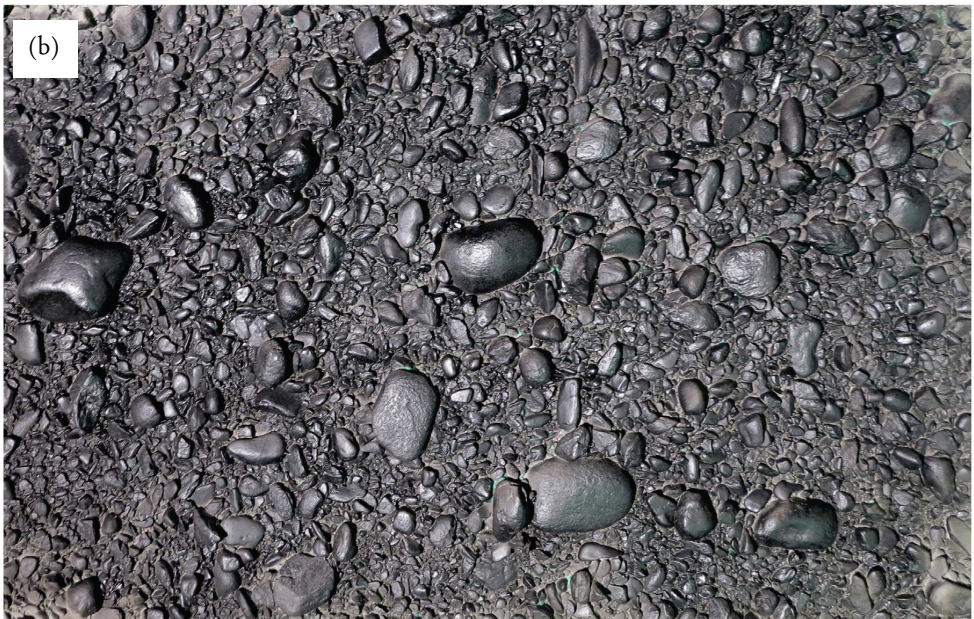
Figure 6: Visual comparison between (a) water-worked gravel-bed surface and (b) its non-porous facsimile.
