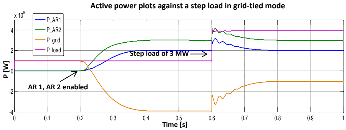
Figure 7-14: Active power plots of AR 1, AR 2, grid and load against a step load change of 3 MW in grid-tied mode
