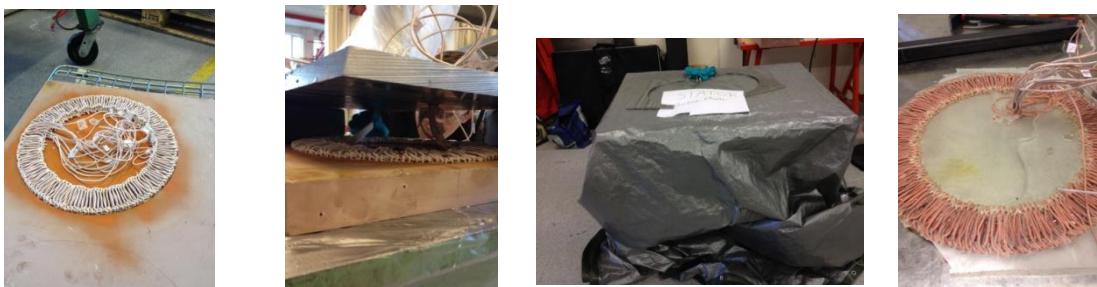
Figure 13 Stator production, open casting
