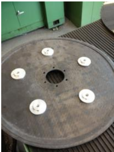
Figure 18 Rotor plate with threaded inserts
