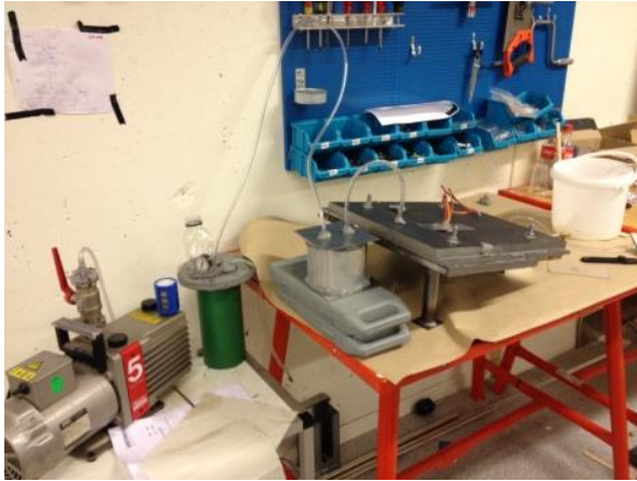
Figure 14 Setup for vacuum casting
