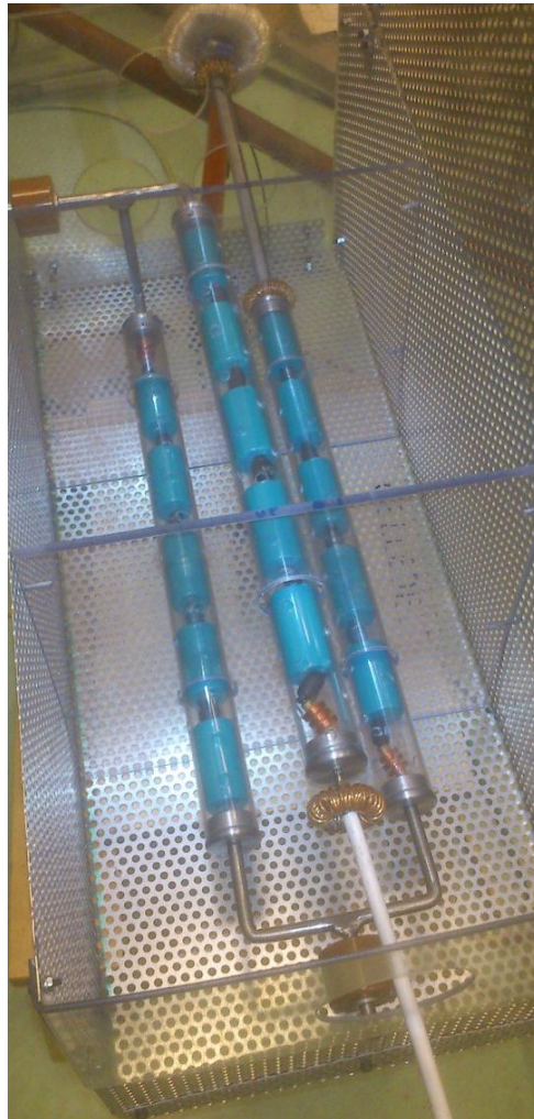
Figure 25. Complete low-pass filter
