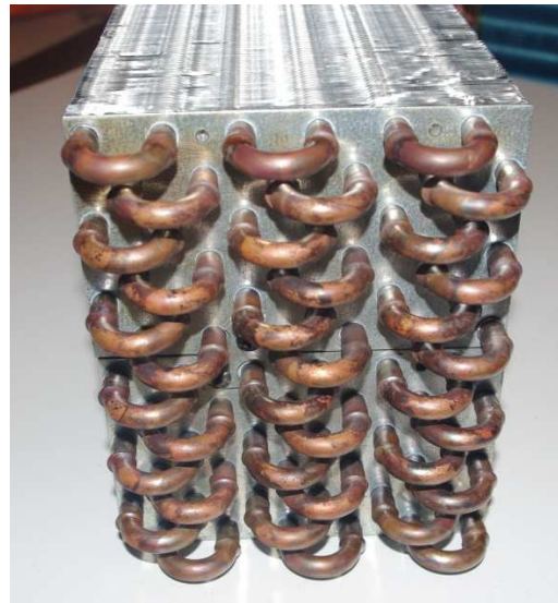
Figure 2.2-10 Main gas cooler #2
