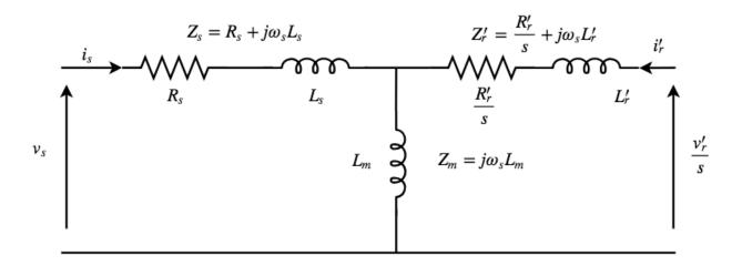
Figure 4.1: Wound Rotor Induction Machine steady-state equivalent circuit
