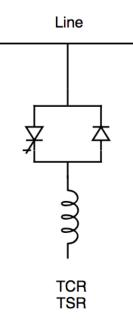
Figure 5.1: Static Var Compensator equivalent circuit
