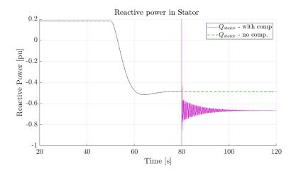
Figure 4.12: Case 3, Scenario 1: Reactive power in stator. Green line - no reactive compensation. Purple line - with reactive compensation.
