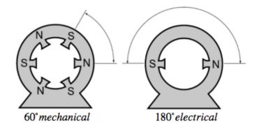
Figure 2.2: Multi- and two-pole machine [16]
