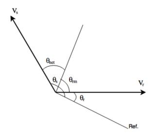
Figure 3.4: Phasor diagram representing the rotary transformer relationships (not scaled) [7]
