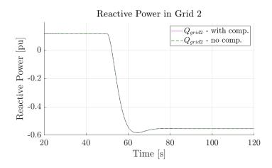
Figure 4.16: Case 3, Scenario 2: Reactive power in grid 2. Green line - no reactive compensation. Purple line - with reactive compensation.
