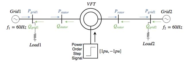
Figure 4.3: Single Line Diagram of the VFT system analyzed in Case 2 Scenario 1
