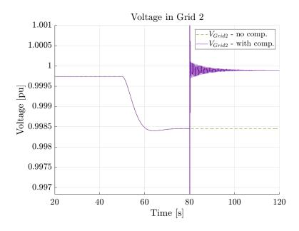
Figure 4.10: Case 3, Scenario 1: Voltage profile in the weaker grid 2. Green, dashed line - no reactive compensation. Purple line - with reactive compensation.
