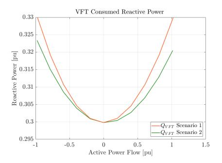
Figure 4.5: Reactive power consumed by the VFT. Red curve is scenario 1 and green curve is scenario 2.
