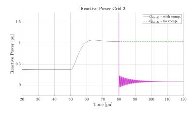
Figure 4.20: Reactive power in grid 2. Green line - no reactive compensation. Purple line - with reactive compensation.
