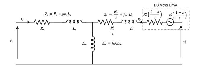
Figure 4.2: VFT Steady-state equivalent circuit [38]
