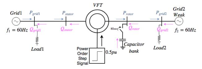
Figure 4.7: Model topology for scenario 1, including power flow direction and placing of the capacitor bank.
