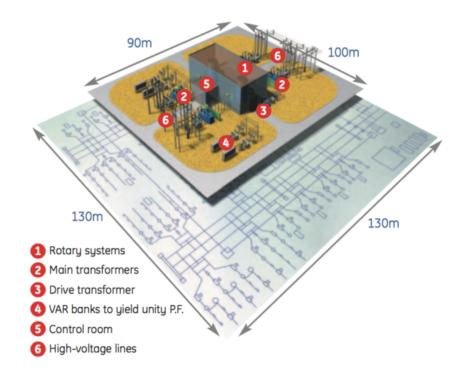
Figure 3.1: VFT substation [27]
