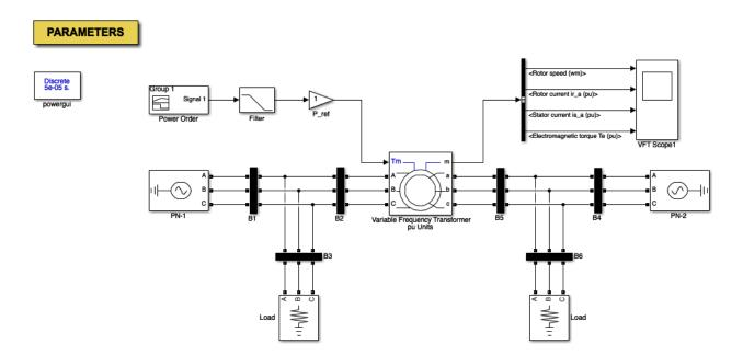
Figure 3.6: The MATLAB/Simulink model of the base case system
