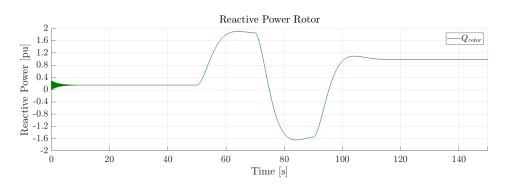
Figure 3.13: Reactive power flow on rotor side.
