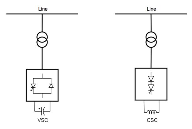
Figure 5.2: Static Synchronous Compensator equivalent circuit
