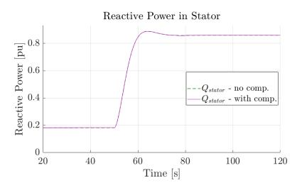
Figure 4.15: Case 3, Scenario 2: Reactive power in stator. Green line - no reactive compensation. Purple line - with reactive compensation.
