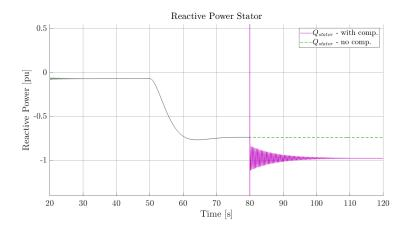
Figure 4.23: Reactive power in stator. Green line - no reactive compensation. Purple line - with reactive compensation.
