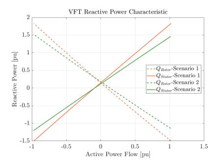
Figure 4.4: VFT reactive power characteristic under varying magnitudes of active power transfer. Red curve is scenario 1 and green curve is scenario 2. Dashed lines represents power in the rotor windings and the solid lines represents power in the stator windings.
