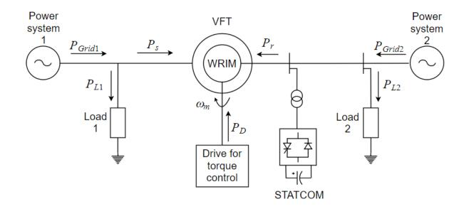
Figure 5.5: The combined system with VFT and STATCOM.
