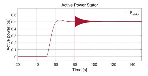
Figure A.2: Case 3, Scenario 1: Active power stator
