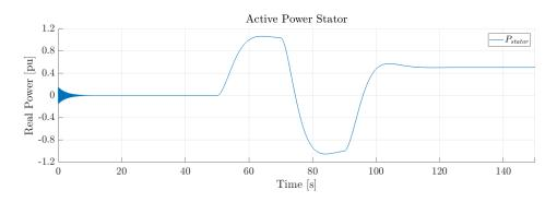
Figure 3.10: Power flow through Stator
