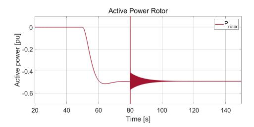
Figure A.4: Case 3, Scenario 1: Active power rotor
