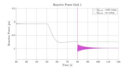
Figure 4.22: Reactive power in grid 1. Green line - no reactive compensation. Purple line - with reactive compensation.
