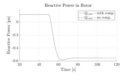
Figure 4.17: Case 3, Scenario 2: Reactive power in rotor. Green line - no reactive compensation. Purple line - with reactive compensation.
