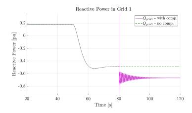
Figure 4.11: Case 3, Scenario 1: Reactive power in grid 1. Green line - no reactive compensation. Purple line - with reactive compensation.
