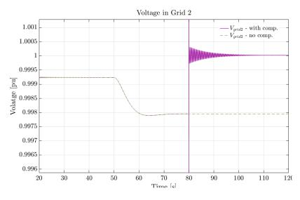
Figure 4.24: Voltage profile in the weaker grid 2. Green, dashed line - no reactive compensation. Purple line - with reactive compensation.
