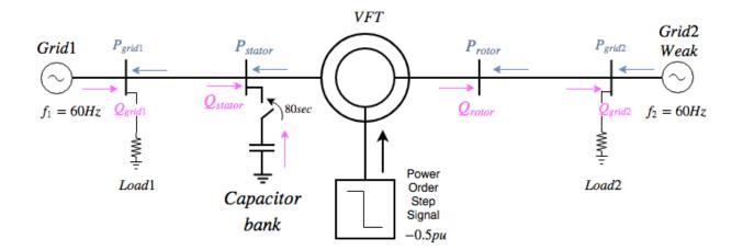
Figure 4.13: Model topology for scenario 2, including power flow direction and placing of the capacitor bank.
