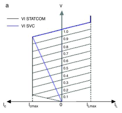
Figure 5.4: The VI-curve of a STATCOM and SVC [46].
