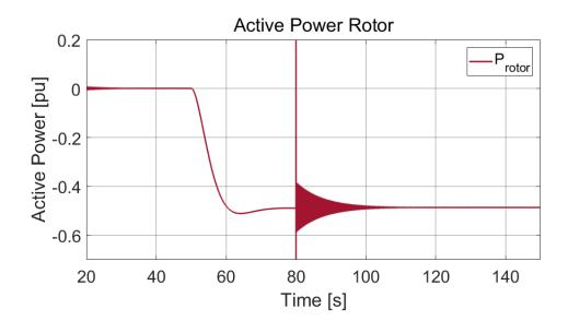
Figure B.4: Case 4: Active power rotor
