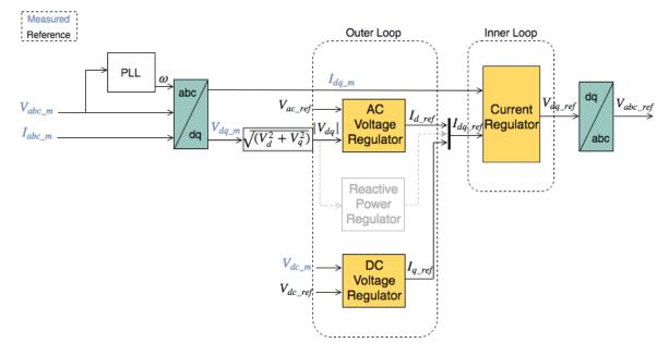
Figure 5.6: General control scheme of a STATCOM
