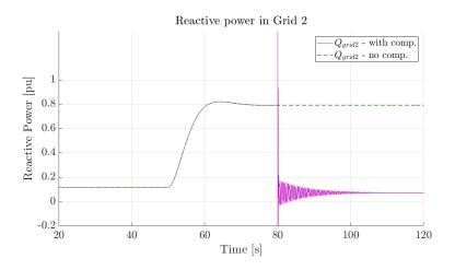
Figure 4.8: Case 3, Scenario 1: Reactive power in grid 2. Green line - no reactive compensation. Purple line - with reactive compensation.
