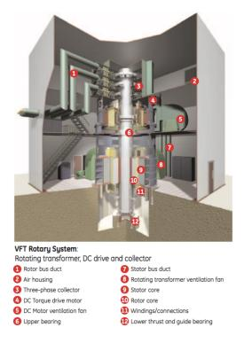
Figure 3.2: System components in a VFT [27]
