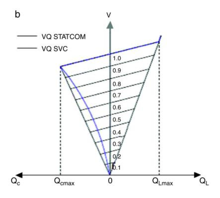
Figure 5.3: The VQ-curve of a STATCOM and SVC [46].
