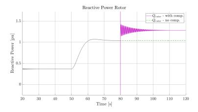
Figure 4.21: Reactive power in rotor. Green line - no reactive compensation. Purple line - with reactive compensation.
