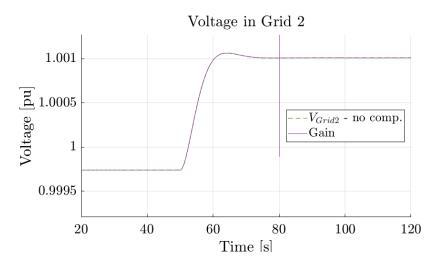
Figure 4.18: Case 3, Scenario 2: Voltage profile in the weaker grid 2. Green, dashed line - no reactive compensation. Purple line - with reactive compensation.
