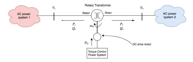
Figure 3.3: Power Flow in a VFT
