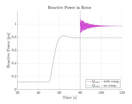
Figure 4.9: Case 3, Scenario 1: Reactive power in rotor. Green line - no reactive compensation. Purple line - with reactive compensation.
