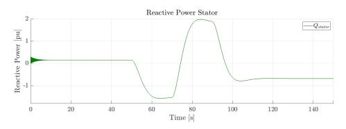
Figure 3.12: Reactive power flow on stator side.
