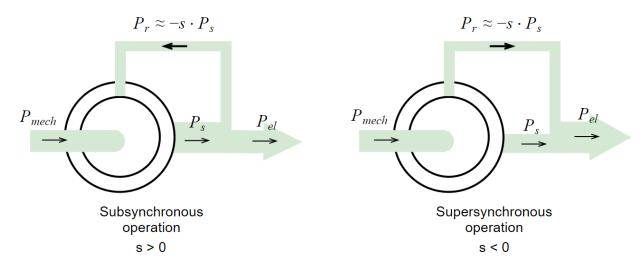
Figure 2.3: Sub-synchronous and Super-synchronous operation of a DFIG [17].  $P_{mech}$  is the mechanical power in the rotor shaft,  $P_r$  is the active power in the rotor windings,  $P_s$  is the active power in the stator windings, and  $P_{el}$  is the total power flowing to the network.
