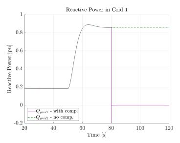
Figure 4.14: Case 3, Scenario 2: Reactive power in grid 1. Green line - no reactive compensation. Purple line - with reactive compensation.
