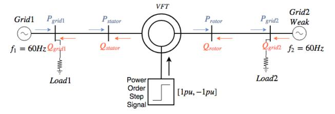
Figure 4.6: Single Line Diagram of the VFT system analyzed in Case 2 Scenario 2.
