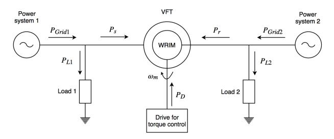
Figure 1.1: VFT System Configuration.
