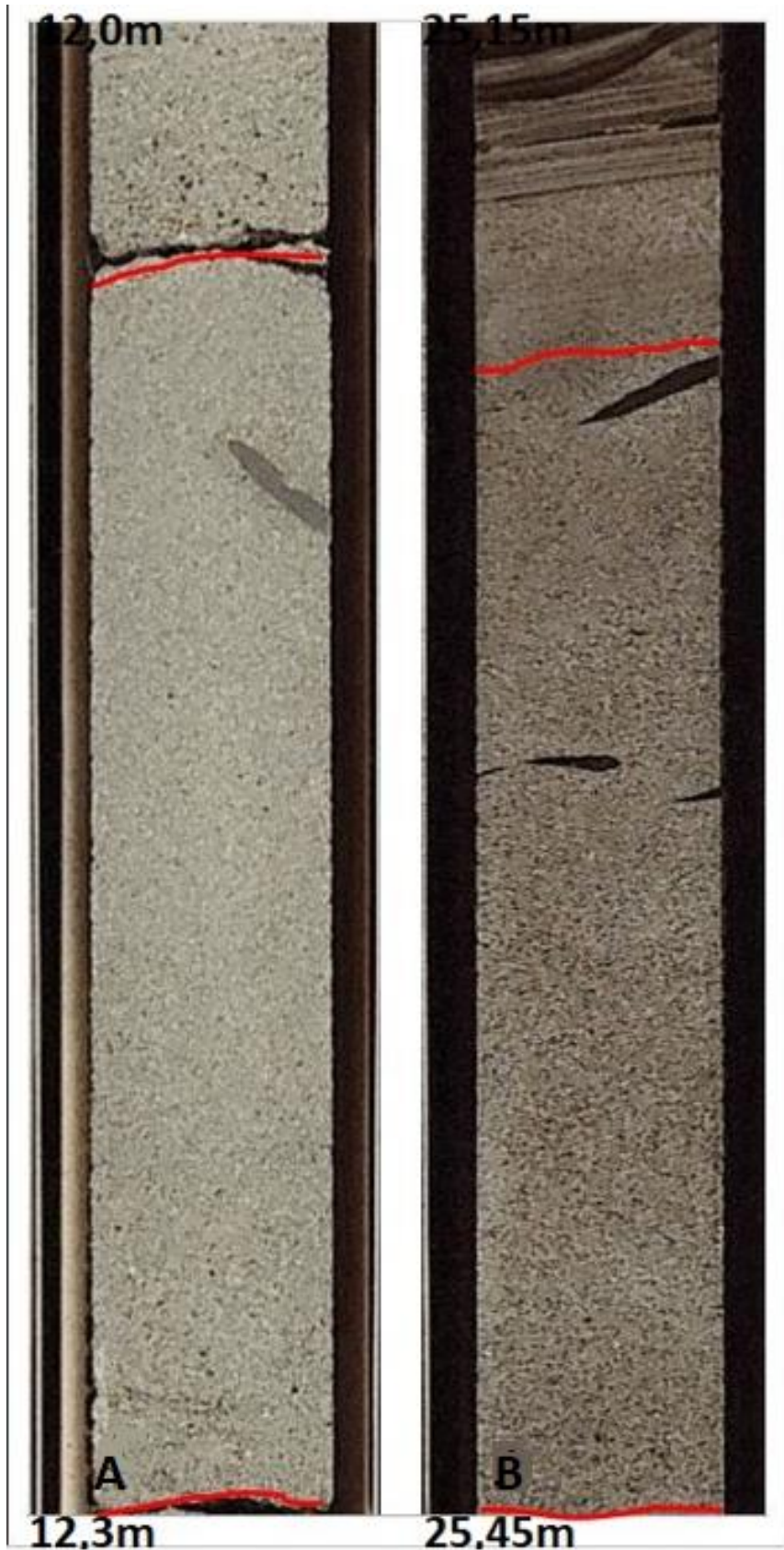
Figure 4.2: Fining up sandstone with clasts (Sst2). The red lines indicates base and top of the lithofacies. A) Clean medium coarse sandstone fining up into fine sand with mud clast at top, from core 6611/09-U-01. B) Coarse sandstone fining up into medium sandstone from core 6611/09-U-02. Horizontally aligned mud clasts in middle and on top.
