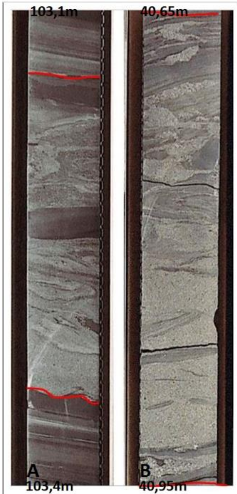
Figure 4.4: Unsorted sandstone (Ds1). The red lines indicates base and top of the lithofacies. A) Mixed sandstone and mud with significant shearing, from core 6611/09-U-01. B) Coarse sandstone and mud in chaotic mix with shearing and sand patches from core 6611/09-U-02.
