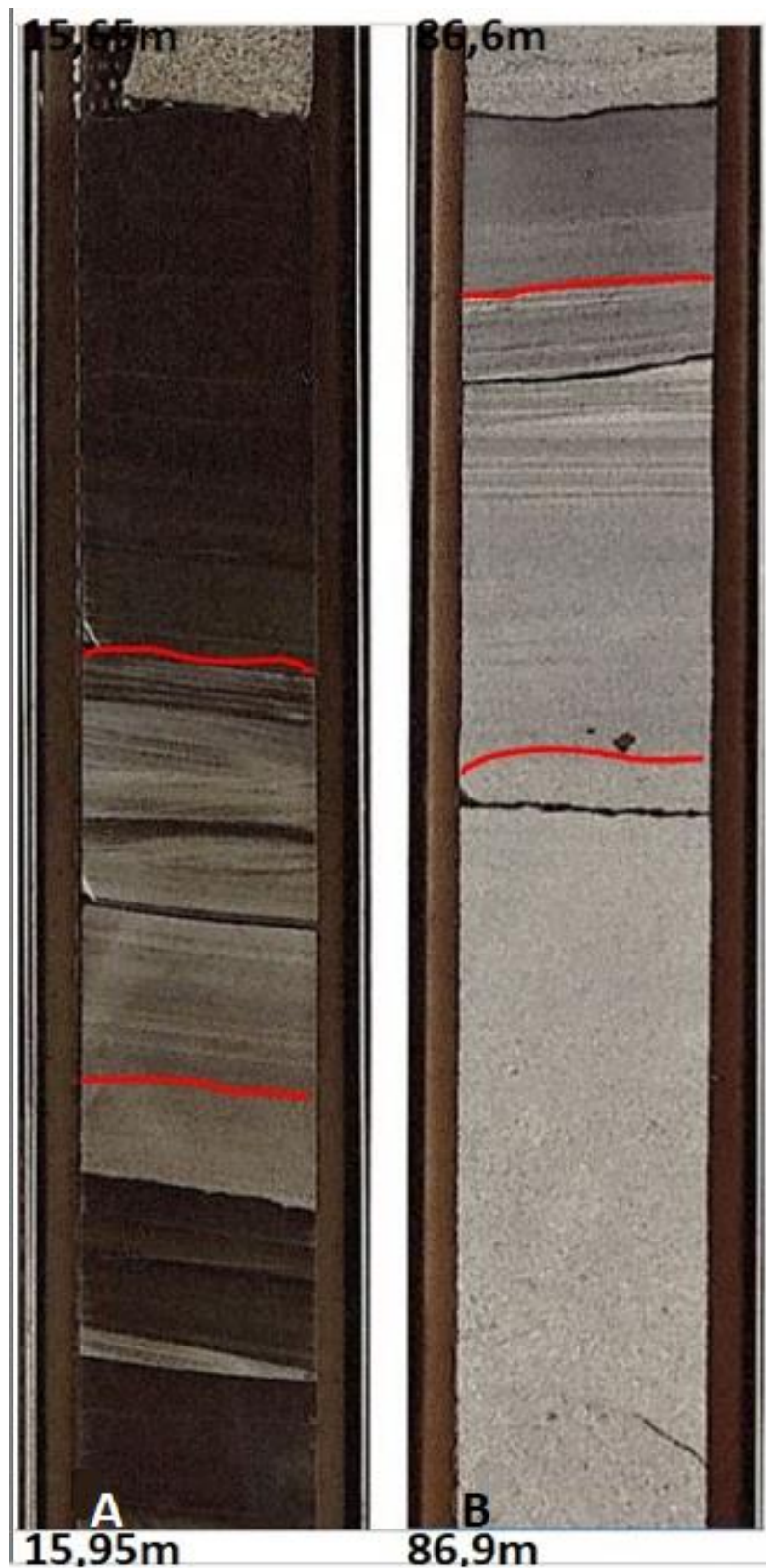
Figure 4.3: Fining up sandstone with current ripples (Sst3). The red lines indicates base and top of the lithofacies. A) Fine sandstone in horizontal lamination at base and current ripples at top from core 6611/09-U-02. B) Very fine sandstone with lamination at base and current ripples at top from core 6611/09-U-01.
