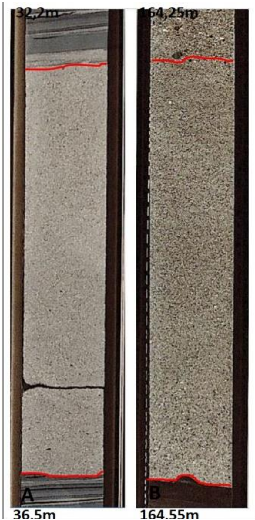
Figure 4.1: Lithofacies clean fining up sandstone (Sst1). The red lines indicates base and top of the lithofacies. A) Clean medium coarse sandstone fining up into fine sand from core 6611/09-U-01. B) Coarse sandstone fining up into medium sandstone from core 6611/09-U-02.
