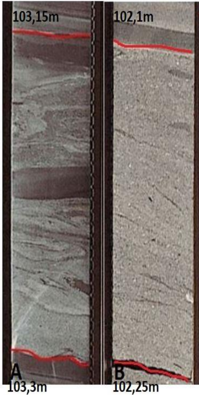
Figure 4.9: Debrite facies association. The red lines indicates base and top (if observed) of lithofacies. A) Debrite with significant mud shearing and clasts (Core 6611/09-U-01) B) Debrite with unsorted matrix and mud streaks (Core 6611/09-U-01).
