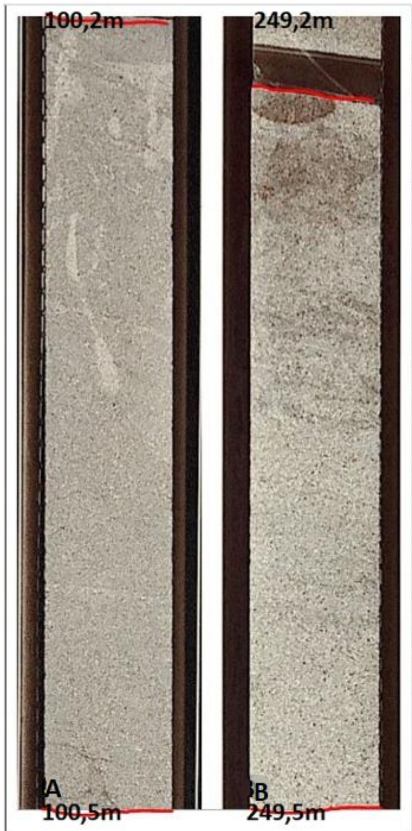
Figure 4.5: Patchy sandstone (Ds2). The red lines indicates base and top of the lithofacies. A) Medium coarse sandstone fining up into fine sand with sand patches at top, from core 6611/09-U-01. B) Coarse sandstone fining up into medium sandstone with sand patches through the bed, from core 6611/09-U-02.
