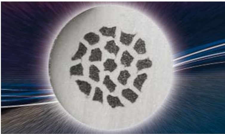
Figure 4.5: Cross-section of superconductor [43].
