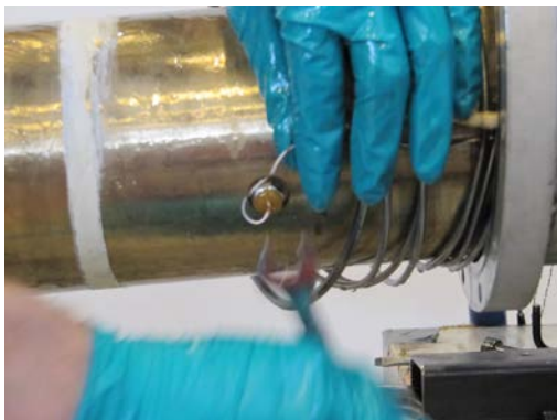
Figure 18: Fixing the temperature sensor
