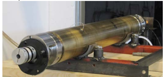
Figure 1: The rotor is fitted inside the stator of drilling machine
