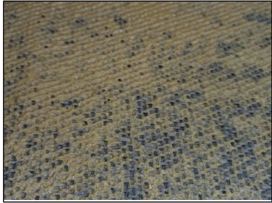
Figure 41: Pictures demonstrating the sludge accumulation on the filter cloth
