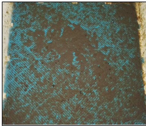
Figure 42: Pictures demonstrating the sludge accumulation on the wedge wire
