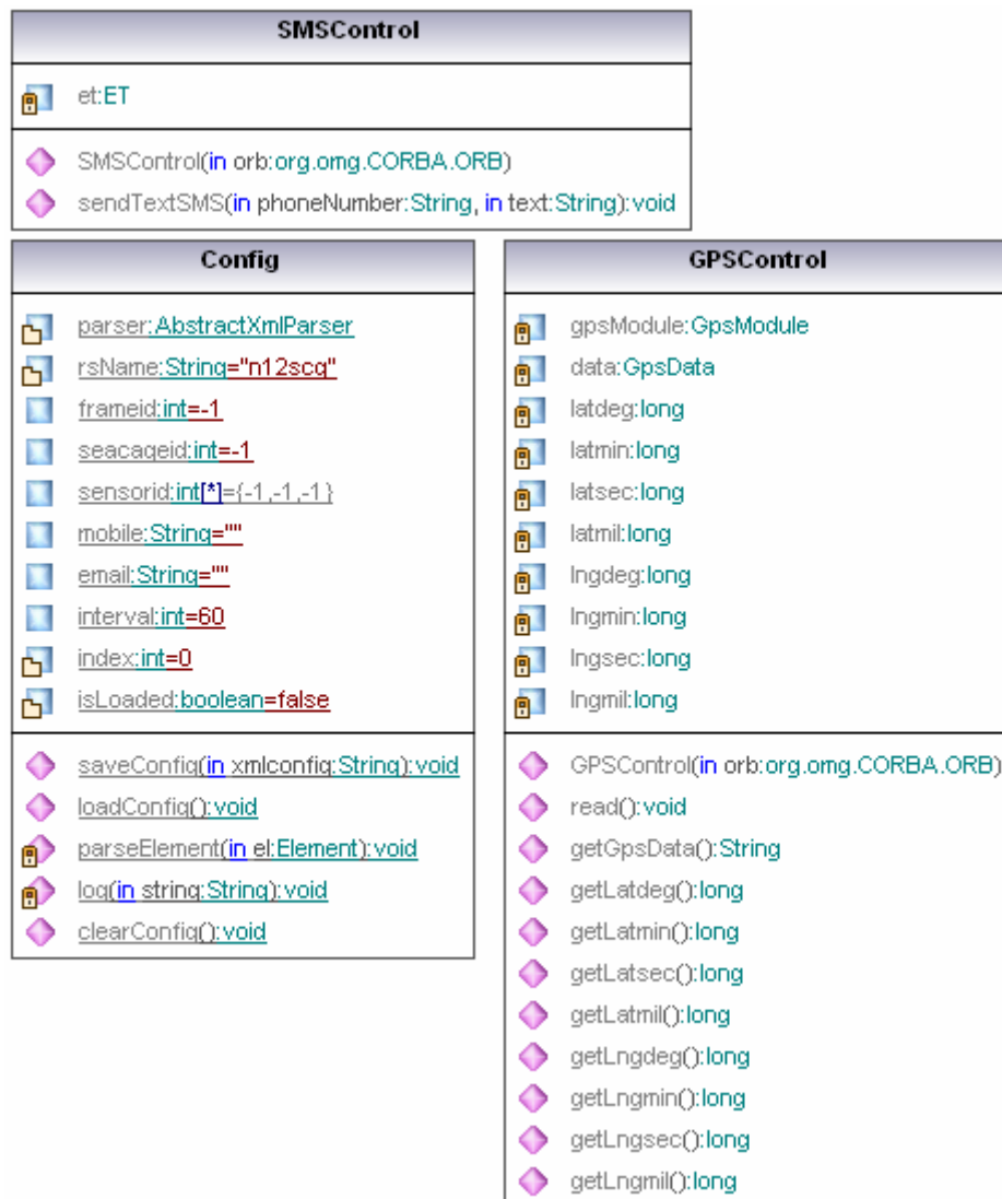
Figure 72: com.telenor.apms.fifamos.n12.utils class diagram
