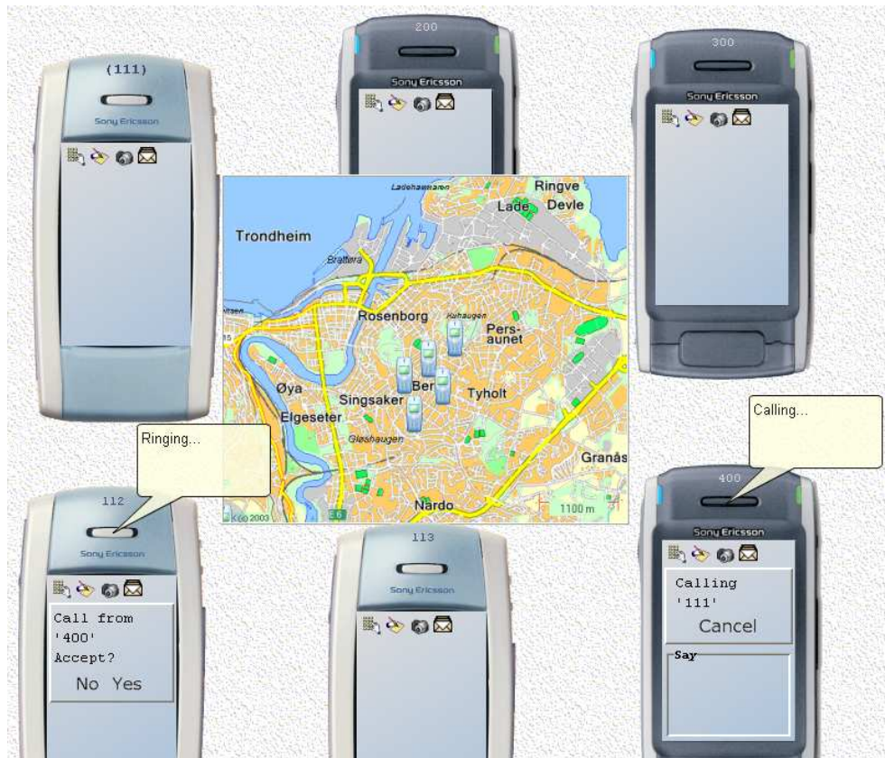
Figure 49: Scenario 3b - Work-related call is made while the subscriber is in the office and no meeting is scheduled at the current time. The call is directed to his desk phone.
