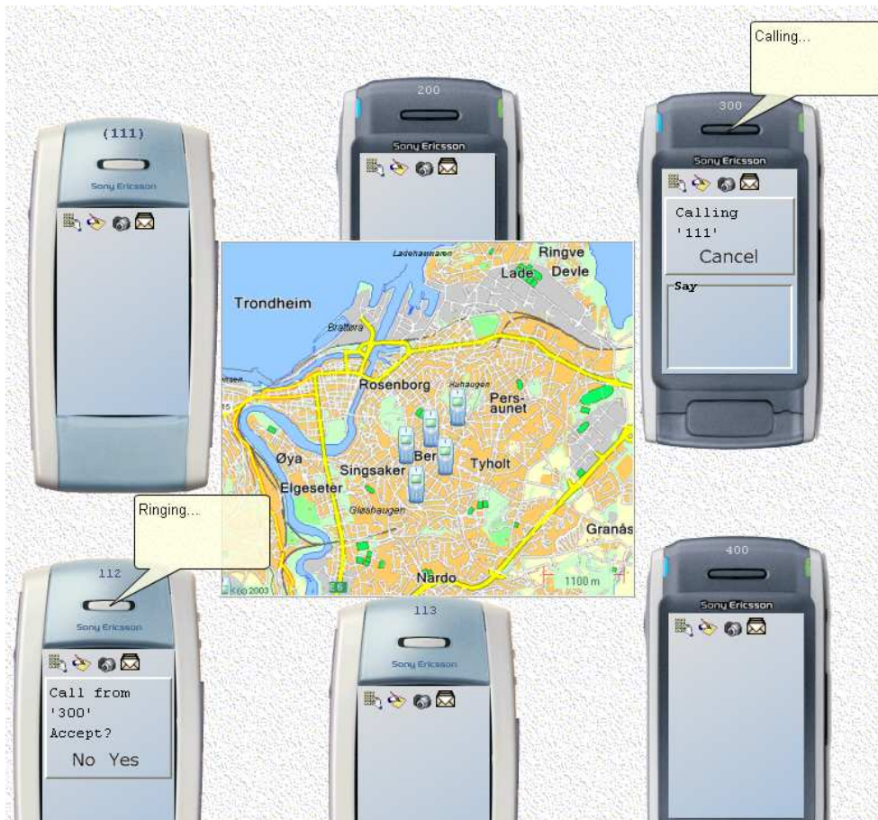
Figure 48: Scenario 3a - Family-related call is made while the subscriber is in the office and no meeting is scheduled at the current time. The call is directed to his desk phone.
