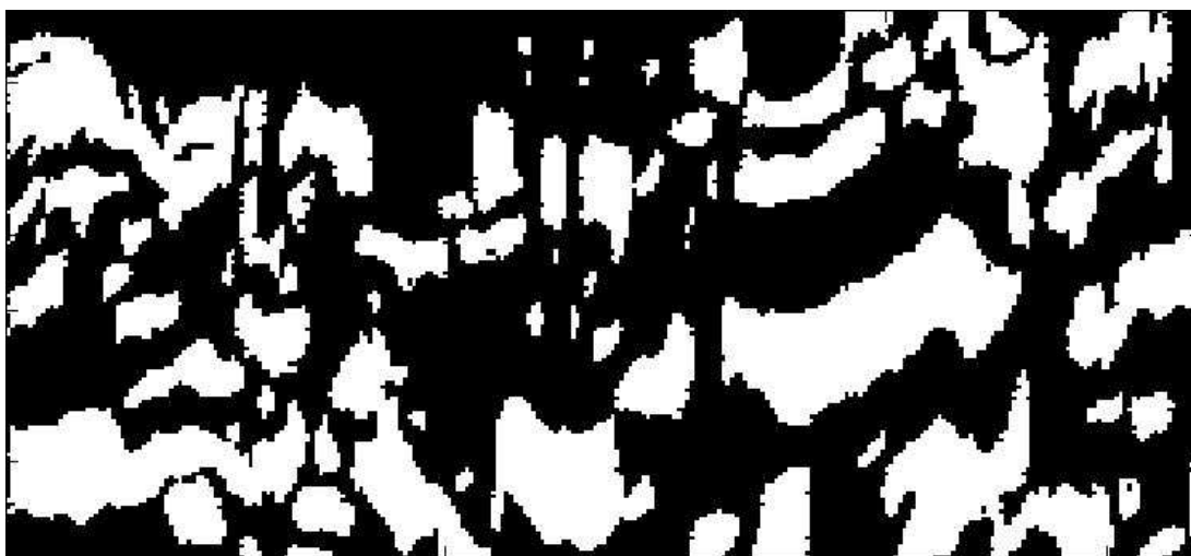
Figure 1: A two dimensional slice of a geological structure where the white fields are shale and the black fields are sandstone. The resolution of the image is 145 \times 271
