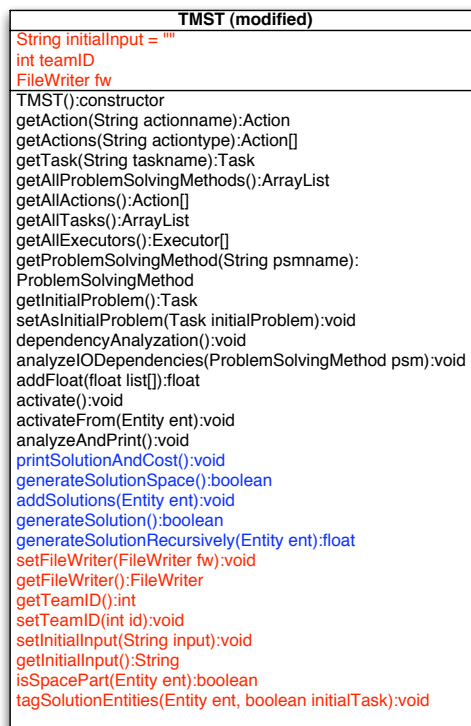
Figure 6.6: A modified UML diagram of the TMST main class. The former version is found in [34]. Red text means new variables/methods in modified classes, blue text means modified variables/methods in modified classes, black text means not modified variables/methods in old classes or variables/methods in new classes.
