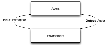
Figure 2.1: An agent in its environment taking as input its perceptions and producing as output its actions, modified from [26].
