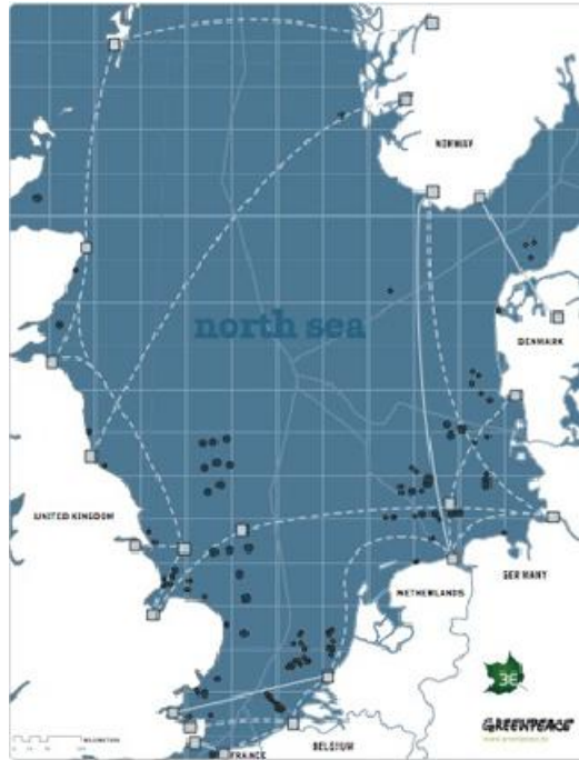
Figure 5-3. One of the alternatives for an offshore power grid in the North Sea (Offshore.no 2008).
