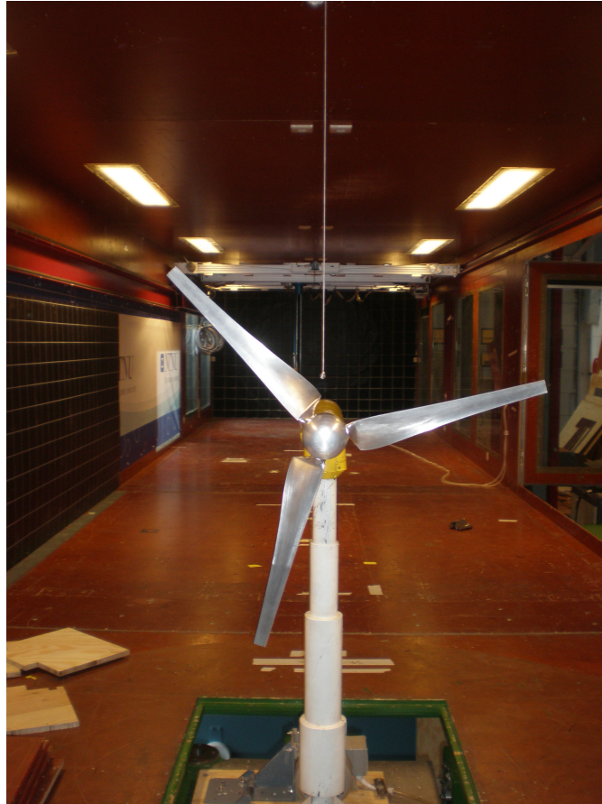
Figure 3.10: Experimental method to place the center of the rotor plane at the center of the balance
