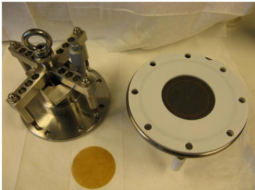
**Figure 3.2:** Sample cell for the IDA system. Top disc to the left
