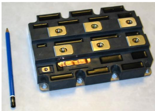
Figure 43 1200 A, 3300 V IGBT module (IGBTs and free-wheeling diodes)
