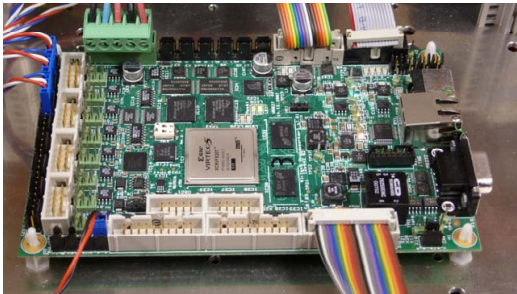
Fig. 11. Processor board based on a Xilinx Virtex FX30T FPGA used for control system implementation in the laboratory setup
