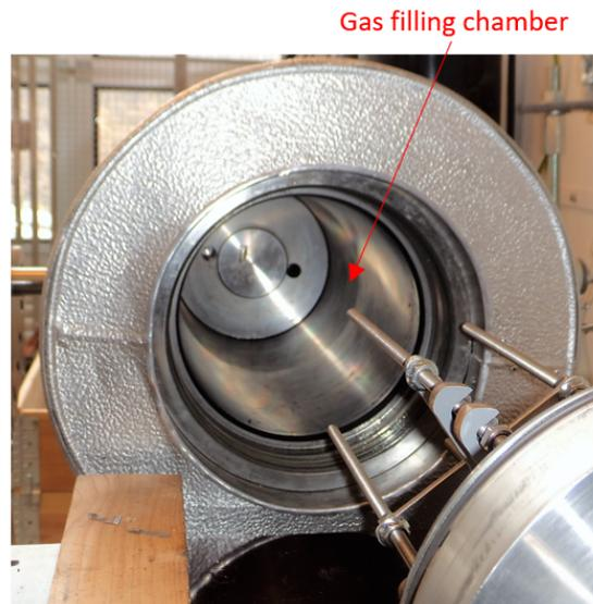
Figure 3.10: Inside chamber of pressure vessel.
