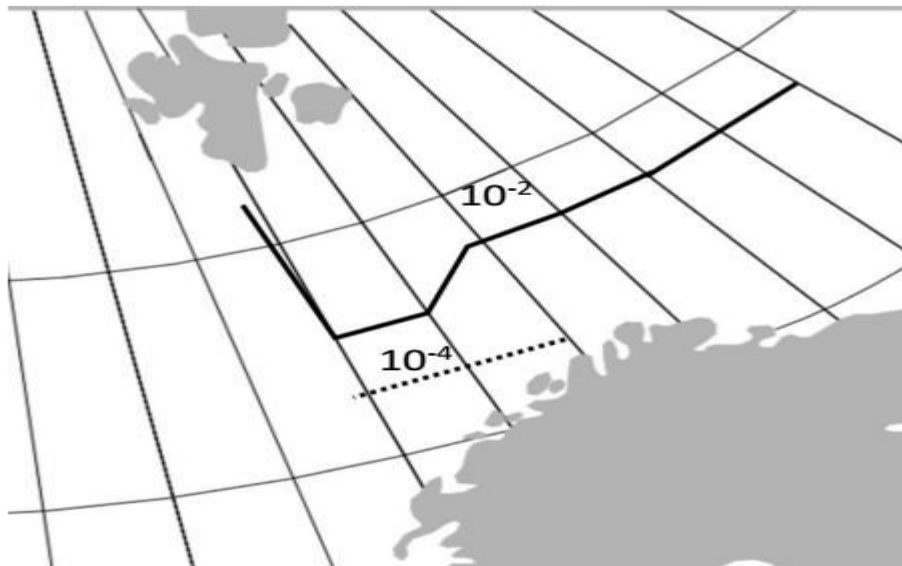
Figure 3 Pictorial representation of probabilistic limits of collision with ice berg (Amdahl 2017)
