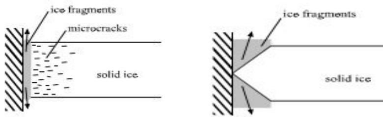
Figure 10 Left picture depicts the case of low velocity impact and the right picture illustrates the case of high velocity impact (Tukhuri, Ice Mechanics-Crushing and Contact 2016)
