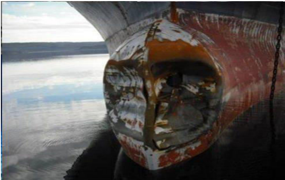
Figure 2 Ship with a damaged bow due to collision with ice berg (Amdahl 2017)
