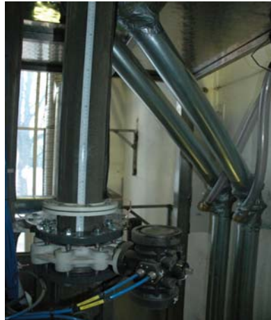
Figure 7.16 - Manual flux measurement in downcomer
