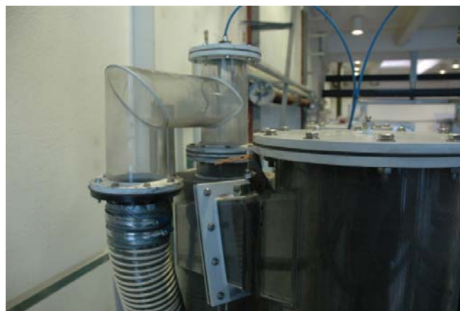
Figure 7.17 - Top of riser and cyclone separator
