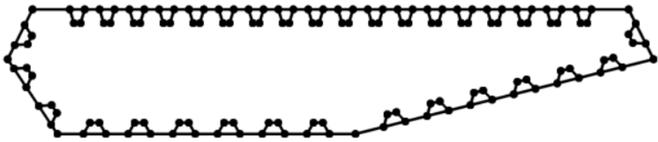
Figure 5.6: Right box girder modelled in Cross-X.
