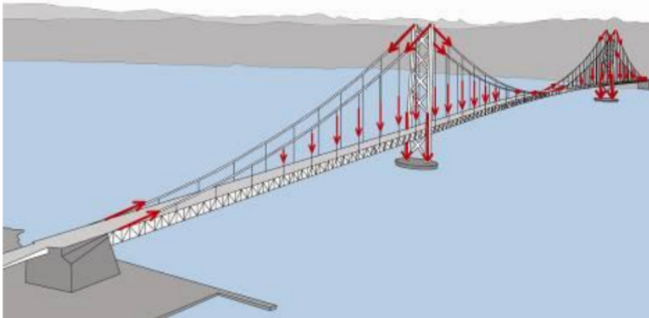
Figure 2.1: Force flow in a suspension bridge [1].
