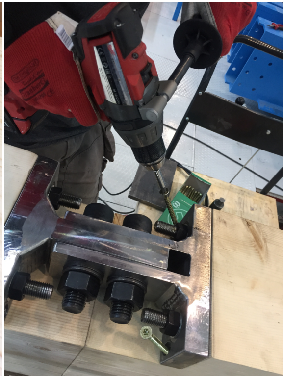
(b) Innskruing med Milwaukee drill
