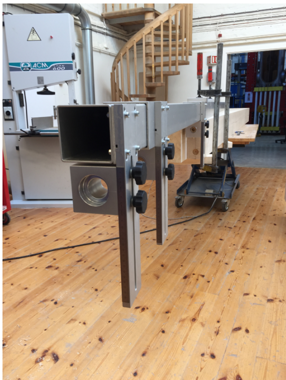
(a) Borrigg plassert for hulltaking
