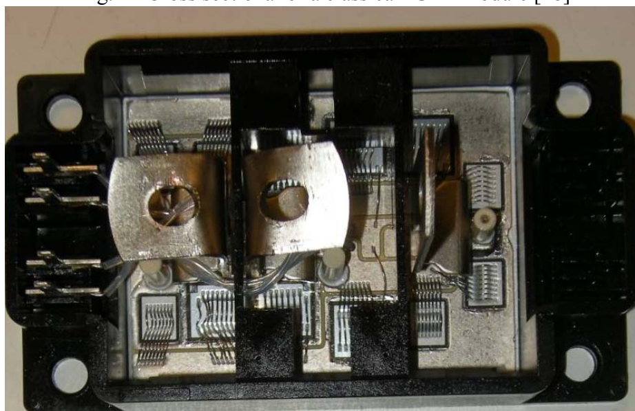
Fig. 13 IXYS IGBT inside (without gel)
