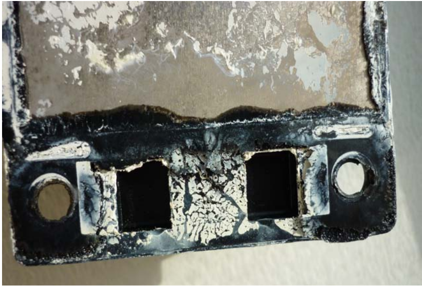
Fig. 36 melted plastic due to temperature out of control
