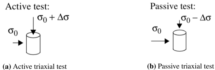
Figure 2.12: Triaxial test to measure active and passive undrained shear strength (Nordal, 2017a)
