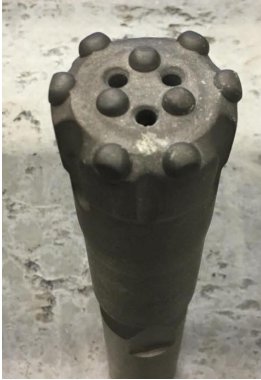
Figur 5.3: Borekrone for hammerboring
