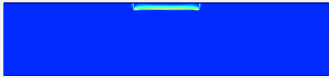
Figure C.21: Failure mechanism for ultimate horizontal loading in the y direction on the longer edge while having \frac{V_{max}}{2} applied
