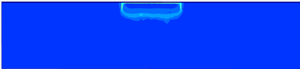
Figure C.23: Failure mechanism for ultimate moment loading in the x direction on the longer edge while having \frac{V_{max}}{2} applied
