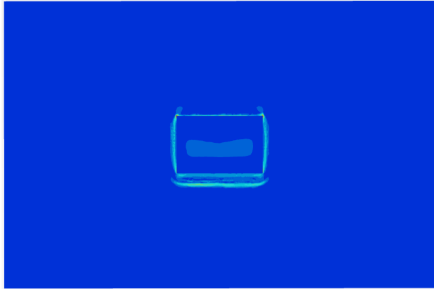
Figure C.37: Failure mechanism for ultimate moment loading in the x direction on the surface while having \frac{V_{max}}{2} and \frac{H_{y,max}}{2} applied
