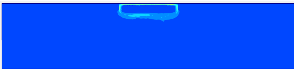
Figure C.13: Failure mechanism for pure moment loading in the x direction on the longer edge
