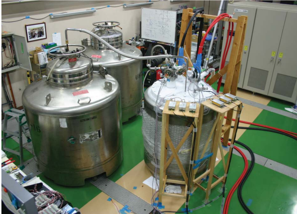
Figure 3.4: The experimental setup in the laboratory. The two left tanks contain liquid helium. The right one contains the superconducting coil.
