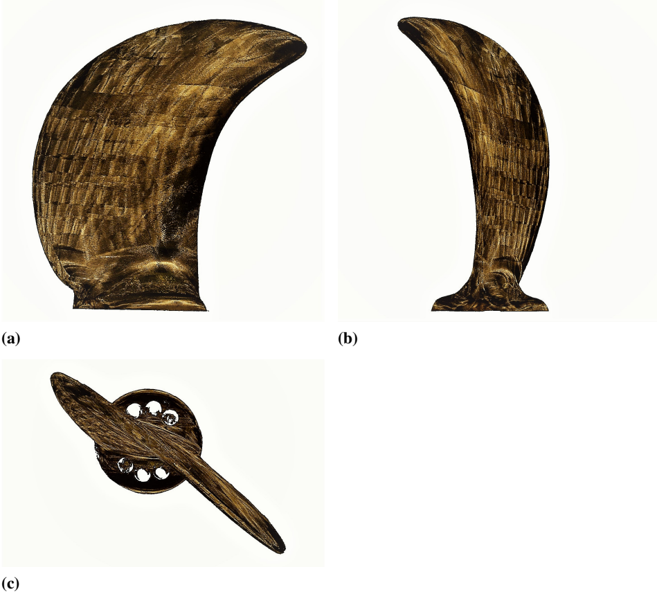
Figure 4.5 The combined point cloud from the scanning process of the blade, which is to be used for the further estimation of design parameters. Some noise has been segmented out manually. Seen from the front (a), side (b), and top (c).
