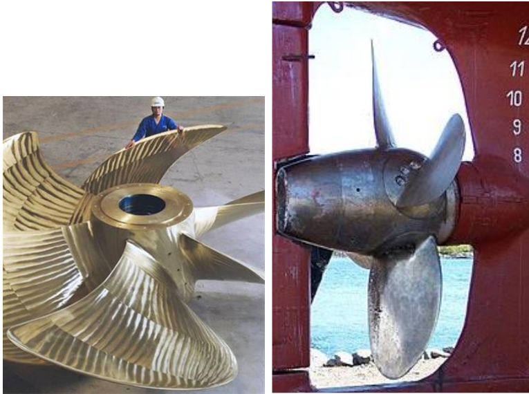
Figure 2.2 Two major types of propellers. Left: Fixed pitch propeller cast in a single piece. Image credit: [37]. Right: Controllable pitch propeller on a Hurtigruten ship. Image credit: [18].
