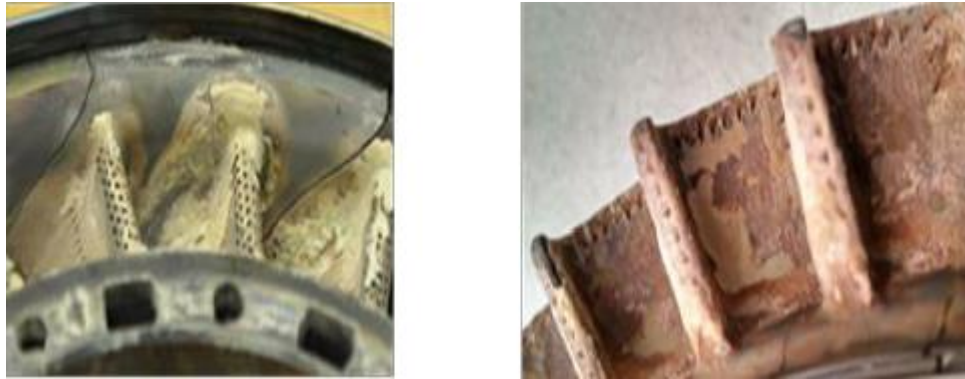
Figure 2: Indications of blade and vane deterioration due to sand and water ingestion.
