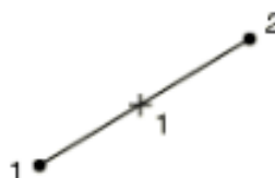
Figur 7.26: T3D2-element; 2 norders stavelement [20]
