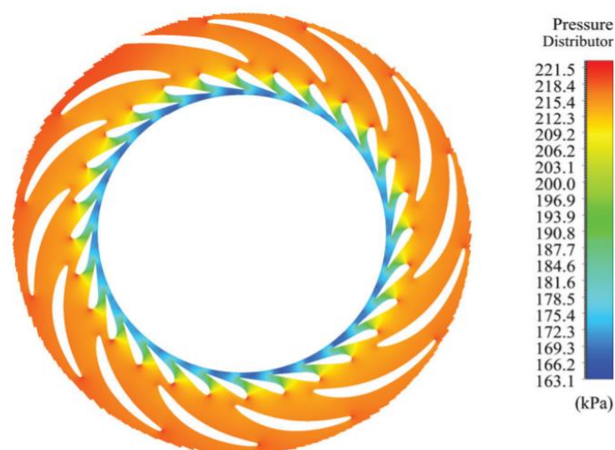
FIGURE 16: STATIC PRESSURE DISTRIBUTION AROUND STAY VANES AND GUIDE VANES, NEGLECTING RUNNER [9]
