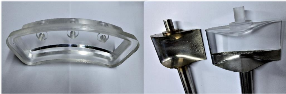
FIGURE 38: CAMERA WINDOWPANE TO THE LEFT, OLD AND NEW GUIDE VANE TO THE RIGHT.
