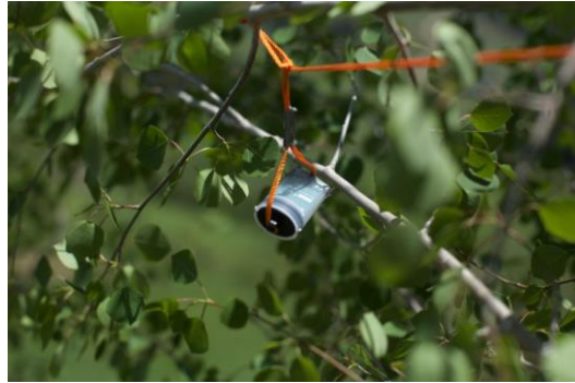
Figure 5 Data logger place in tree canopy with sensors orientated upwards.
