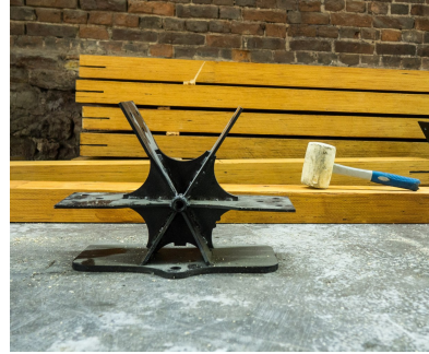
Figure 2.14: Joint used in the Wooden Geodesic Dome in St. Petersburg, [10].
