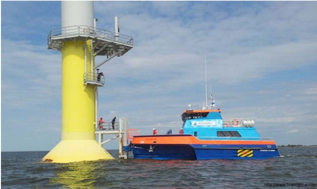
Figure 1.2: SWATH-type CTV During a Transfer Operation
