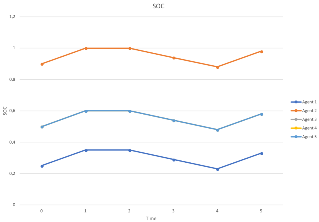
Figure 5.31: SoC level for all agents in a hierarchical-distributed operation model without congestion
