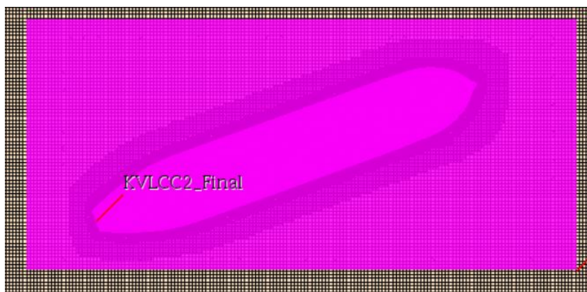
Figure 7.27: Size of the inner domain with the obliquely oriented vesse, oblique wave simulation
